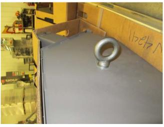
2. Align the tower with the base. Be careful not to pinch electrical cords. Do not lower all the way onto the base. Lower the tower far enough to thread the cords into the tower.
